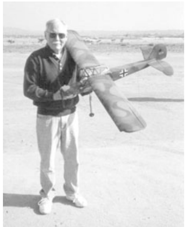
Don Wemple and his Fieseler Storch. Powered by a Sp 600 with a 3:1 gear box and 8 2000 cells.
