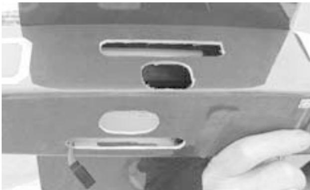
Camera ports were cut into the fuselage for either a directly down shot or an oblique shot to the right.
