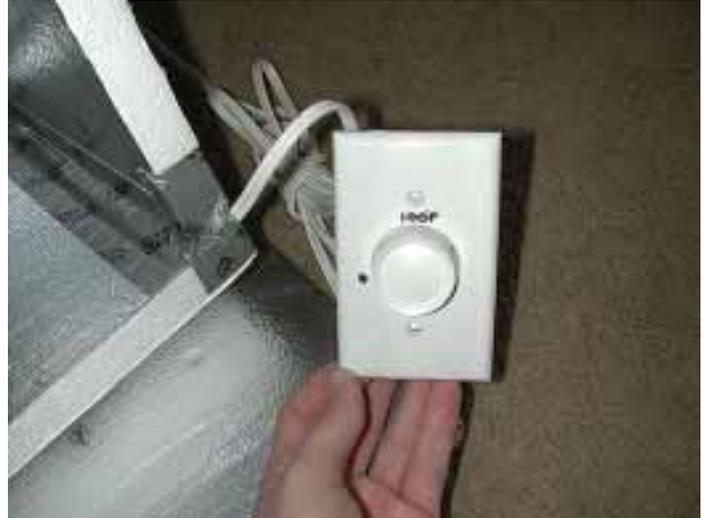
**2. Dimmer switch control.** Temperature of oven is controlled by adjusting the voltage to the lamps.
