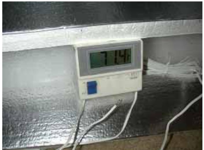
**3. Thermistor readout.** Simple digital thermometer with thermistor probe located inside oven.
