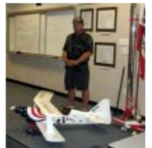
22 x 10 prop. The plane does all full-house aerobatics and can fly for 20 minutes on one charge. The plane weighs about 12 lbs. and makes almost 2,000 watts of power.
