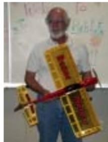
Chuck Grim showed off his new Mini Lazer 3-D. He flies it using a Razor 2500A motor, 4.4 x 1 gearbox, on 8-950 mah cells. The all up weight of the plane is 20.5 oz.
