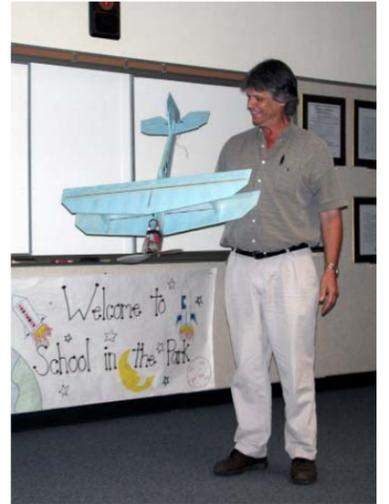
Mike Morgan brought his new custom foam bi-plane. The wings are constructed of blue foam and have no airfoil at all. Mike says that the model is very predictable and could actually be used as a trainer. He flies it with a Li-Po battery and brushless motor and gets about 30 minute flights.
