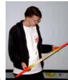
David Fee showed an unfinished hollow-molded F5D wing. The span is 40" and the airfoil is quite thin—only 6.4%. The skins are a glass/balsa/glass sandwich, with carbon reinforcements in high-stress areas. The spar caps are carbon, but are still a little too flexible because of the limited thickness of the wing.
