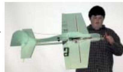
Mike Blott also brought his tiny EDF-50-powered Optica model. It is constructed mainly of foam, and should be presented as a construction article in an upcoming national hobby magazine. Mike is now using a 2-cell 540mAh lithium polymer pack, and the flight times have increased to 10 minutes! This is an impressive small, light model.
