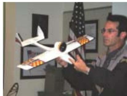
Mike Blott showed a Wattage Turbo Hawk which has recently been given a new lease on life. The well-used plastic fuselage has been repaired with polyurethane glue, which Mike reports bonds to the plastic better than
