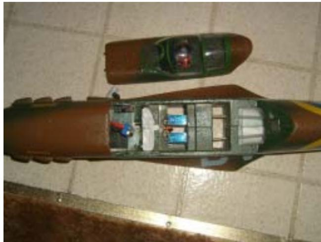
On Off switch inside and larger battery area to receive the 1500 3 cell lipo.
