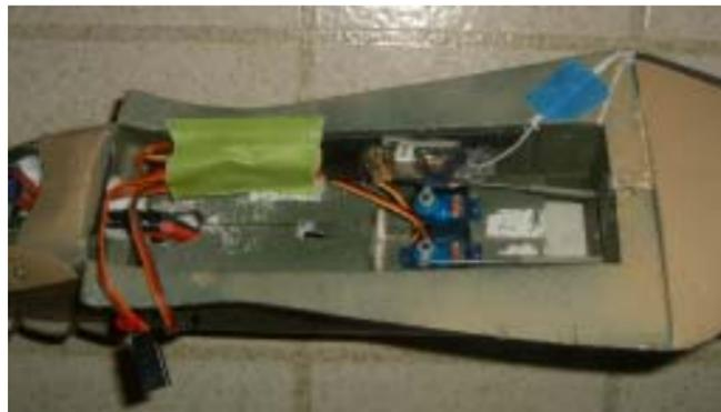
RC Direct 5 channel Berg receiver and two Hitec 55's
