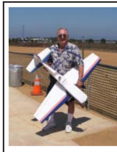
Ray Fulks holding a 19 % scale model of a Staudacher S-300. It was built 4 yrs ago for E use from an Ace kit. It is powered by two 3S4P Thunderpower LiPo 7800 packs in series connected to a Sculze 55 bo ESC. An Aveox 1412 2 Y motor swings an APC[E] 15x8 prop. It will perform the IMAC Sportsman aerobatic sequences. It will do this routine for three 8 min flts on one charge
