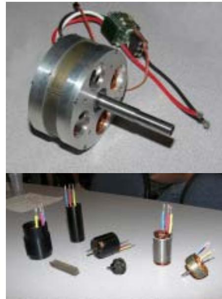
from the floor. He highlighted his new ORK 19-series 24-slot, 8-pole motors. These are high torque motors intended for direct drive in planes or geared in helicopters. Steve's motors have Si-steel laminations which are stamped in India, while the stator stacking and winding is done in Mexico. The neodymium magnets are made in China but motor design, development, assembly and testing (and repair) are all done in Rancho Bernardo, CA.
