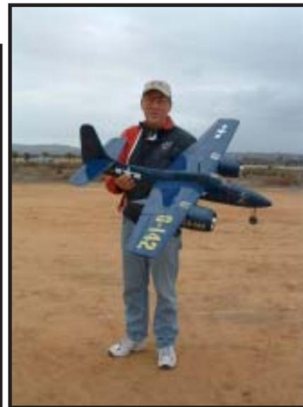
I just finished this TigerCat F7F-3 for Steve Neu. It's a fiberglass fuse and built-up wing and tail with Spring-Air retracts added plus the usual panel-lines, nomenclature etc.... Weight w/o motors or batteries is 3.4 lbs. Finish is paint and Monokote. Frank
