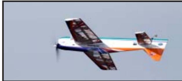
**Wingspan** : 1,540 mm (60.62 Inches) , **Length** : 1,570 mm (61.81 Inches), **Main Wing Area** : 46 sq dm2 The motor is a Hacker C-50 10L with a gearbox using a Castle Creations speed controller running a 18x10 prop using Neu batteries 6S 4900
