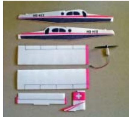
actuators. The 90 mAh li-poly battery has two small magnets that click onto two corresponding magnets on the receiver. The motor is a 7 mm, 3.3 ohm pager motor. This is a great radio for peanut scale r/c models (something I had been dreaming of for many, many years).
