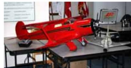
on scale taxi lights and a super sanitary job of hiding the E-Flight 160 outrunner into the scale radial engine turning an 18X 8 prop. The model is powered by a (2) 5S 5200 Lipo packs and includes the Robart retractable landing gear made for this model. Frank reports the Beech weighs just 18 lbs which is a lb less than suggested for glow power!
