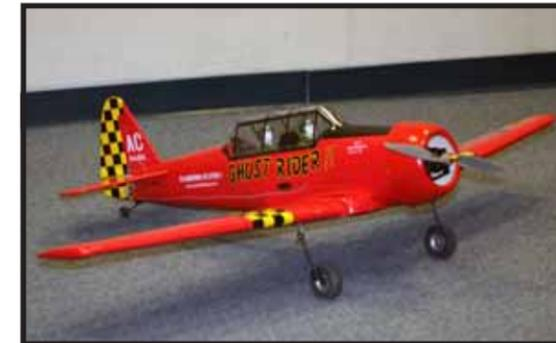
AT-6 modified from a VQ Warbirds ARF designed for .40 to .60 glow but readily modified to a NEUMOTOR 1910-2Y and 4S4300 Lipos. Phil was able to slip the batteries onto a fuel tank shelf and move the servos aft for the extra room required. The Texan came in at just 6 lb., 2 oz with retracts and a fancy
