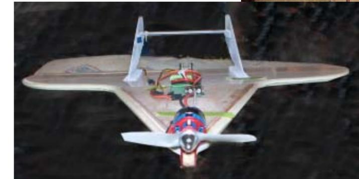
54 AMP. Castle Thunderbird, servos; High Tec Hs 55 & 56 , amp draw; static: 47, pressurized by blower: 34 (sym. .. 90 mph) on the ground. It sure would be a kick to test it in a wind tunnel.
