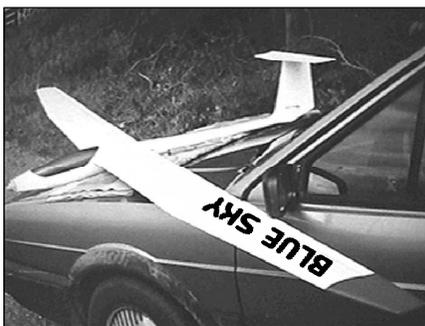
It is his own design and, of course, scratch built. Wingspan is 3.5 meters, weight: 3600 grams, motor: Keller 35/10, 15 1700 mAh
