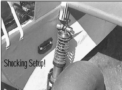
these ambiguously named planes. His even has R/C car-type shocks mounted for stabilization during those high speed ground runs. Power is an A15 on 12 cells. Mike says it's easier to build than the Lazy Bee but it is not a very speedy, Speedy.
