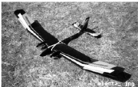
This is a TWIN Electra with 2 Astro FAI05's on 16 cells (600ma scr). From the DEAF www site.
