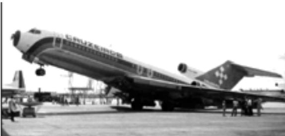
This Boeing 727 was without any weight in the front (seats, galleys or fuel). Then, the engines weight pushed the tail to the ground. May 1982.
